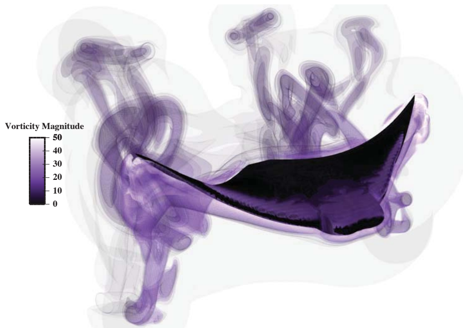
Figure 1. Wake structures around a cownose ray, visualized via isosurfaces of the Q -criterion, colored by vorticity magnitude.
